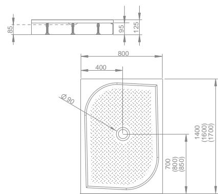
To install direct on basement or with front panel, siphone outlet Ø 90 mm, installing legs included, recommended siphons TB 90P, R400 SLIM.
