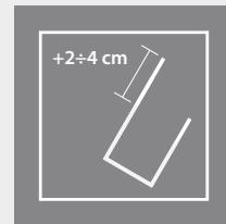
Wall profiles with adjustment to compensate for wall irregularity
