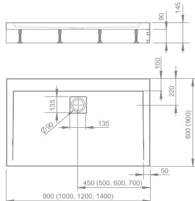
Aluminium panel with chrome or white colour finish, a Ø 90mm hole for a siphon, recommended siphon: R399. When ordering a shower tray, please select the variant of panel.
