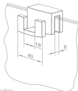
Usefull hanger intended to fix on the glass in profileless cabins
