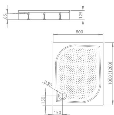
To install direct on basement or with front panel, siphone outlet Ø 90 mm, installing legs included, recommended siphons TB 90P, R400 SLIM.
