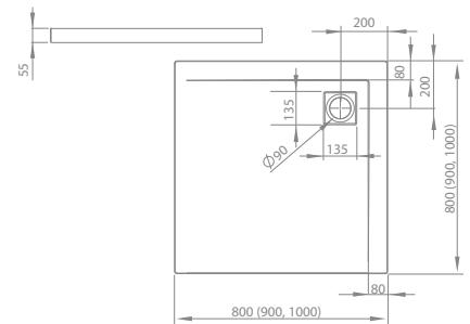
Aluminium panel with chrome or white colour finish, a Ø 90mm hole for a siphon, recommended siphon: R399. When ordering a shower tray, please select the variant of panel.
