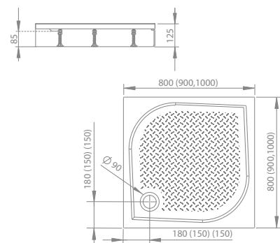
To install direct on basement or with front panel, siphone outlet Ø 90 mm, installing legs included, recommended siphons TB 90P, R400 SLIM.
